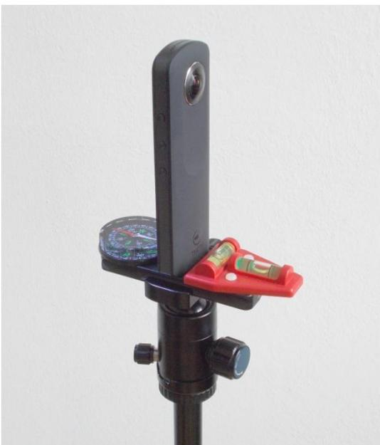
*A simple leveling plate turns the Theta S into a powerful full-sphere surveying tool. With a two-way bubble level the camera is vertically aligned for the exposures. On images shot with this setup, the horizontal coordinates of celestial objects, light pollution domes, horizon lines etc. can be measured directly.*
