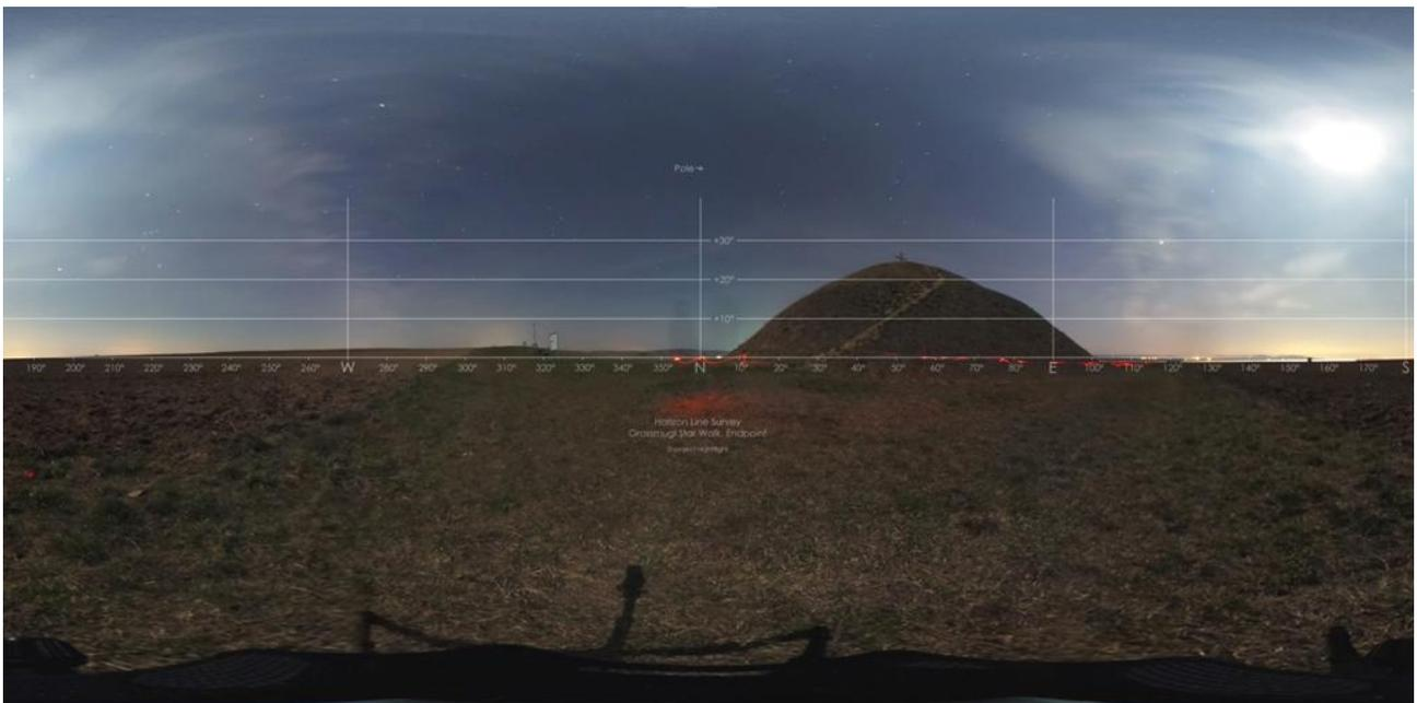
*Equirectangular image of an observing location in moonlight at the endpoint of the Grossmugl Star Walk. In the image, coordinate lines of the horizontal system (azimuth, height) were added in Photoshop. Exposure of the original Theta S image was 60 seconds at ISO 100.*
